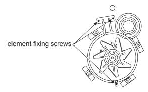
Remove 2 screws from the top of the element and 1 from the bottom of the element in side the oven. Lift element out carefully, disconnect the terminals connected to the element noting their positions. If it is not possible to disconnect the leads in this way, pull cooker forward to gain access to the rear, remove screws securing the electric cover to the back sheet and remove cover and disconnect the terminals from the rear.
